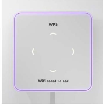
As soon as the LED ring turns white, the WPS is activated and it will contact the router.
