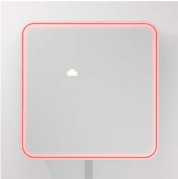
This means that the CO<sub>2</sub> values are above 1200 ppm → ventilation is necessary.
